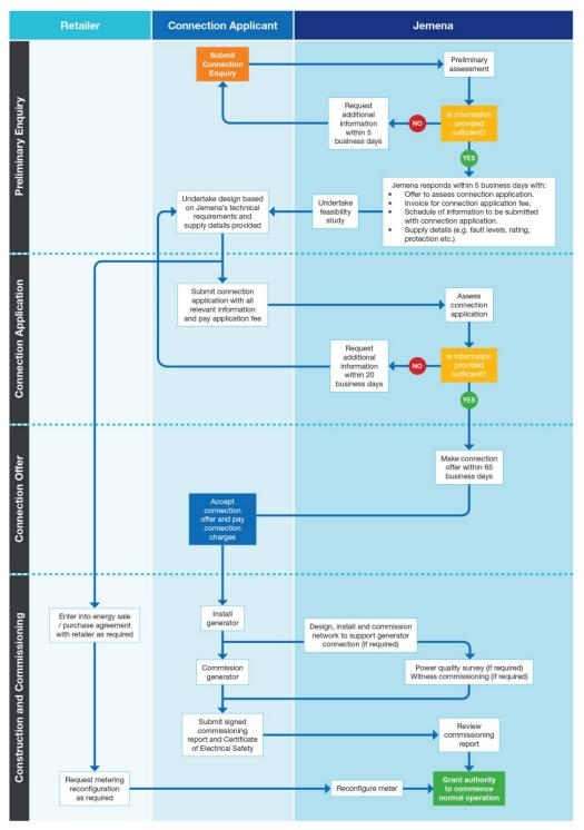
Figure 3–1: Negotiated connection process for embedded generators
