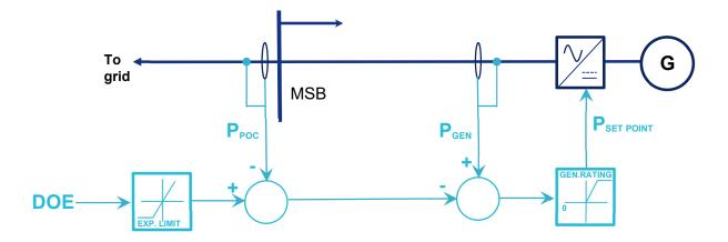
All values above are in kilowatts. The control diagram for the above is illustrated below.
