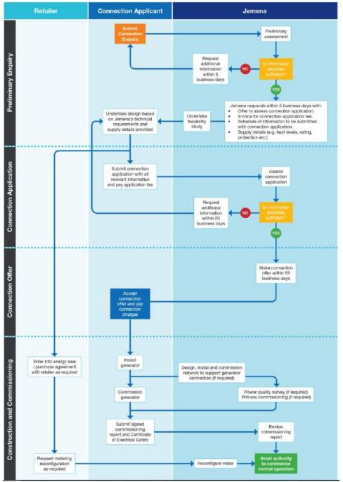
Figure 2–1: Simplified connection process for IES (30 kVA – 200 kVA)
