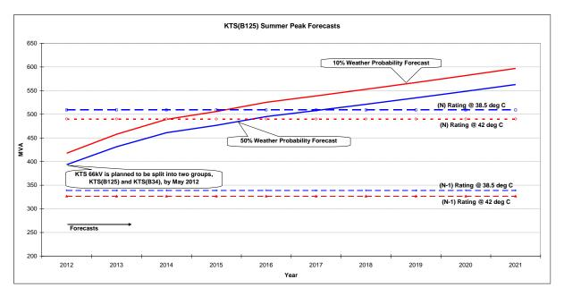
Figure 6: 10<sup>th</sup> and 50<sup>th</sup> percentile summer maximum demand forecasts KTS B1, B2 and B5 transformer group
