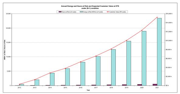
Figure 1: Energy at risk at KTS for the 50<sup>th</sup> percentile demand forecast
